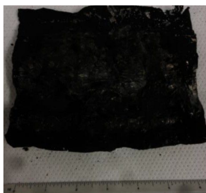
Figure S2. Photograph of a 6-inch CNT-Al structure synthesized in a 1-inch furnace.
